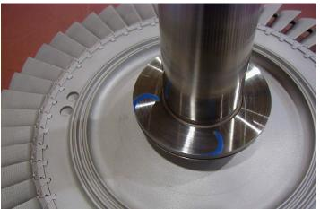
Repaired & rebladed rotor ready for installation
