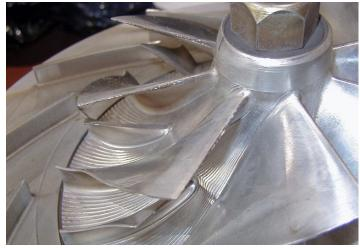
Air end impeller installed & ready for final assembly
