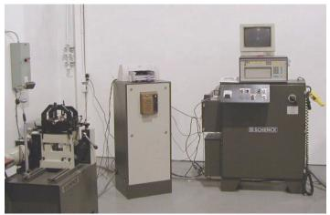
Small component balancing center for rotors up to 100 lbs
