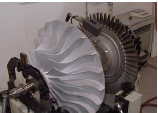
Repaired rotor ready for balancing
