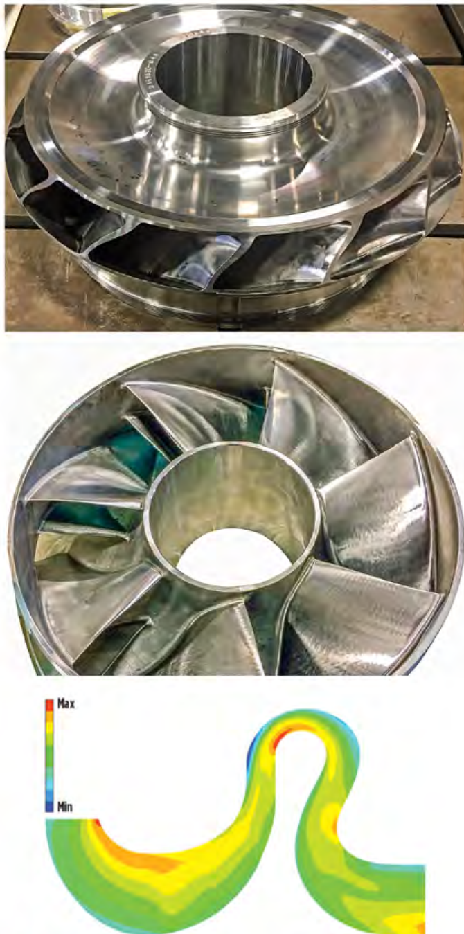
FIG. 4. View of the very-high-flow, mixed-flow impeller (top and middle) and the circumferentially averaged meridional distribution (bottom).
