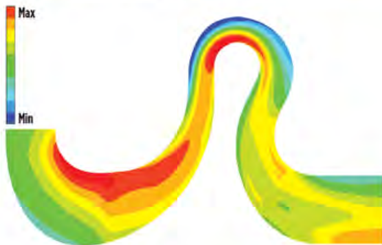
FIG. 2. Original design of the very-high-flow impeller (top), with circumferentially averaged meridional distribution (bottom).
