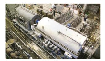
**Figure 5.** Full-load test of MR and C3 compressors with gas turbine and 12 MW electric motor.
