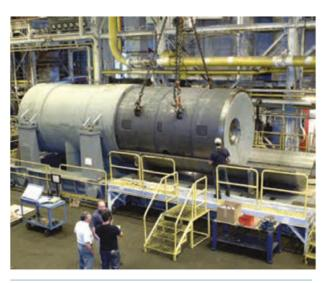
Figure 4. Removing the inner barrel of an Elliot 88MB mixed refrigerant compressor.
