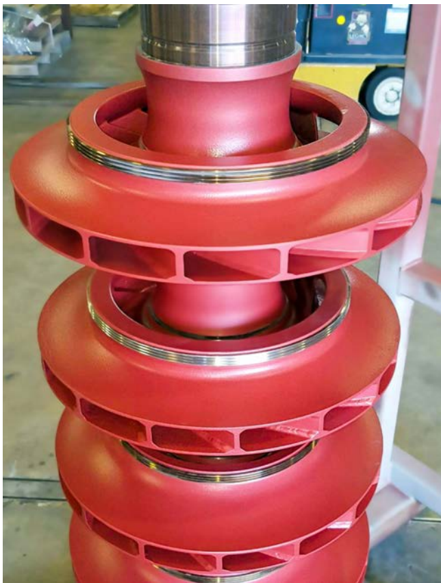
Figure 3. Elliott specialty Pos-E-Coat® hydrogen compressor coating.
