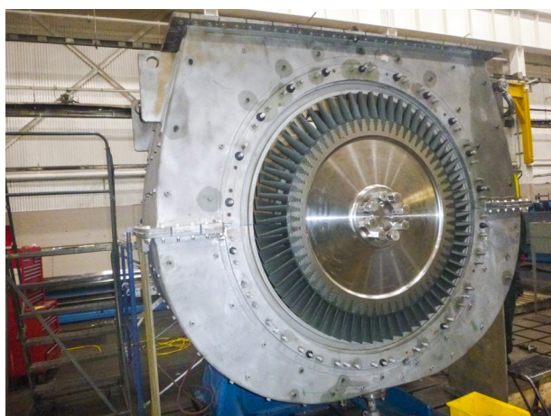
Figure 5. Cleaned and partially reassembled TH-100 expander.
