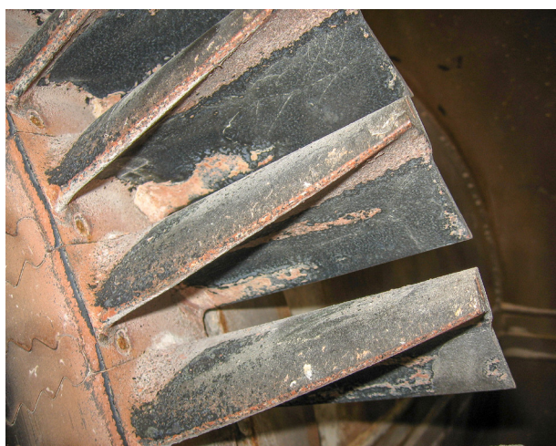
Figure 3. TH-100 rotor blades as received after the first five year run.
