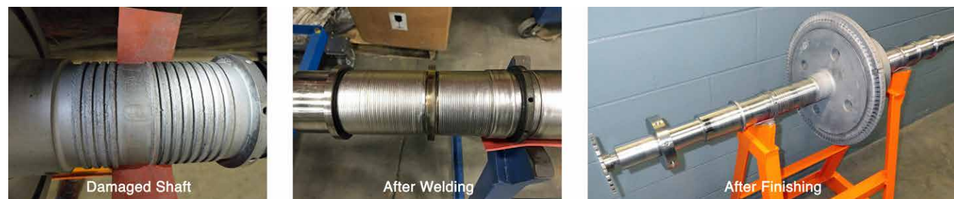
FIGURE 6 Shaft Damaged by Extensive Pitting
