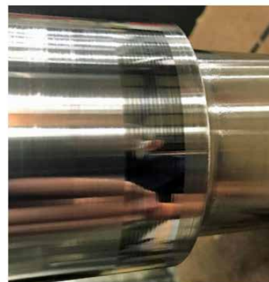
FIGURE 7 Example of a Burmished Probe Area after Repair (left). The repair region appears dark because of a difference between the base and weld metal; however, the repair met the geometric tolerances, surface finish, and electrical runout (right) required for a probe area.
