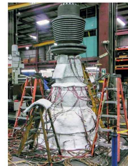
FIGURE 4 Post weld heat treatment setup.
