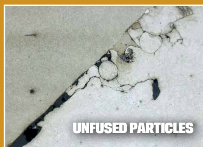
FIGURE 3 Typical defects that occur in laser welding. These defects were found in a weld made using powder based filler metal delivery. Porosity can be seen speckling each image.
