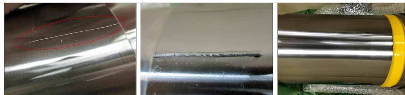
FIGURE 8 The scratch (circled) in a journal area (left); the same scratch after LBW repair (middle); and the repaired area after final machining (right).
