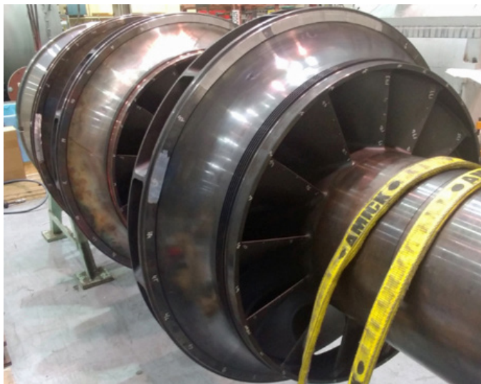
Figure 2. Rotor assembly of the selected impeller wheel.
