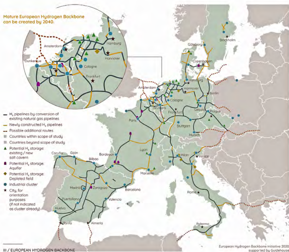
Figure 1. Plans for European Hydrogen Backbone by 2040 (with permission from the European Hydrogen Backbone Initiative). 3
